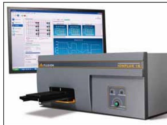
**Figure 1.** The IonFlux system utilizes a “plate reader” format to simplify workflow and increase throughput. Systems are available with 16 and 64 amplifiers. Throughputs of 10,000 data points per day can be achieved. It integrates a temperature control module, which enables the user to perform temperature dependent electrophysiology assay screening.
